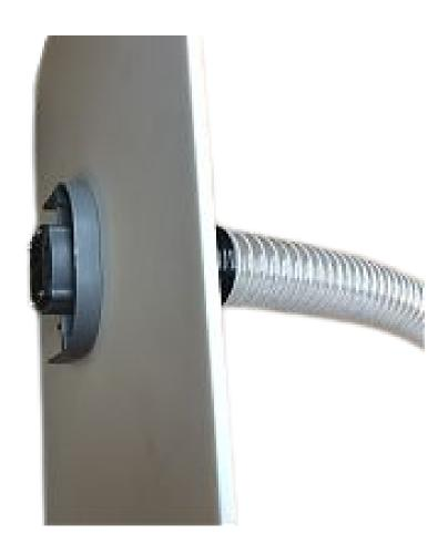
Attach one end of hose to the flange installed on the interior.
