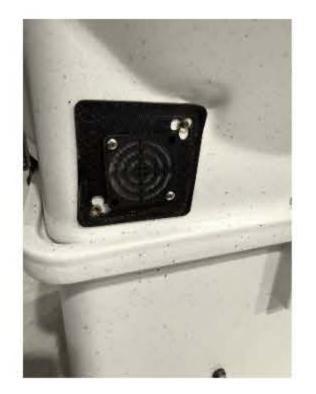
Remove old air intake housing and leave the filter and gasket in place
