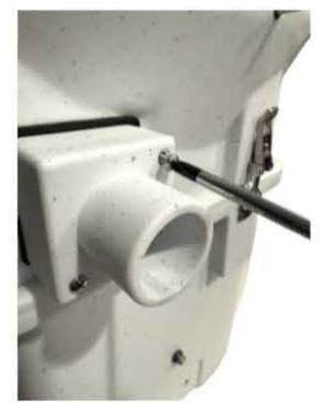
Loosen and remove the two screws that hold the old airintake housing on.
