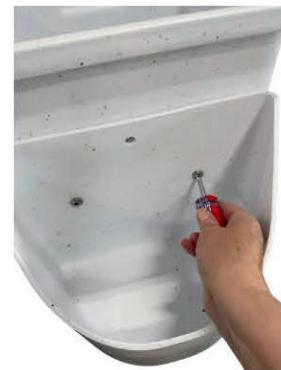
Remove the 3 phillips head screws that secure the bottle holder to the base. Set the 3 screws to the side for later use.
