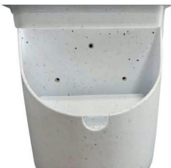
Place the new bottle holder in front of the base and align the holes with the 3 brass inserts on the front of the base. Carefully thread each screw from the previous bottle holder into the inserts by hand. Then tighten each screw evenly with a screwdriver, until tight.
